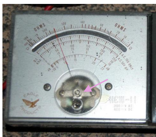
Figure 10 Adjusting screw to reduce zero error
