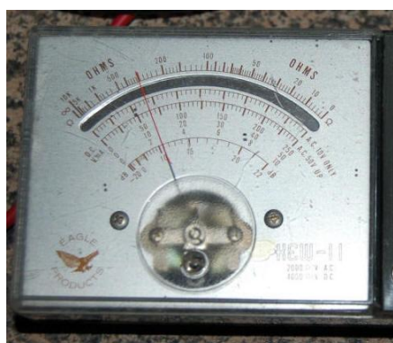
Figure 8 A mirror to reduce parallax error
